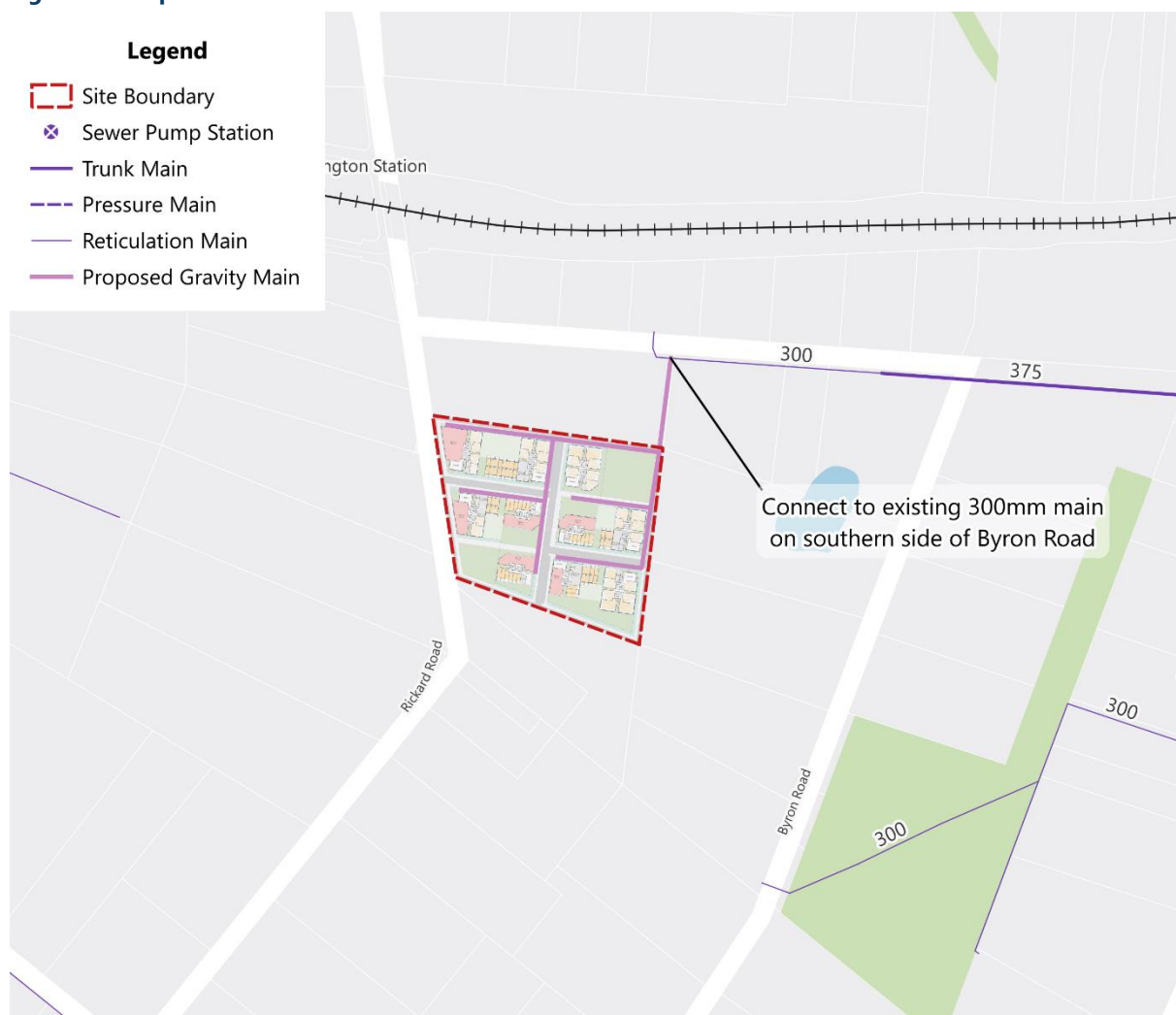
Figure 6 - Proposed Sewer Infrastructure
