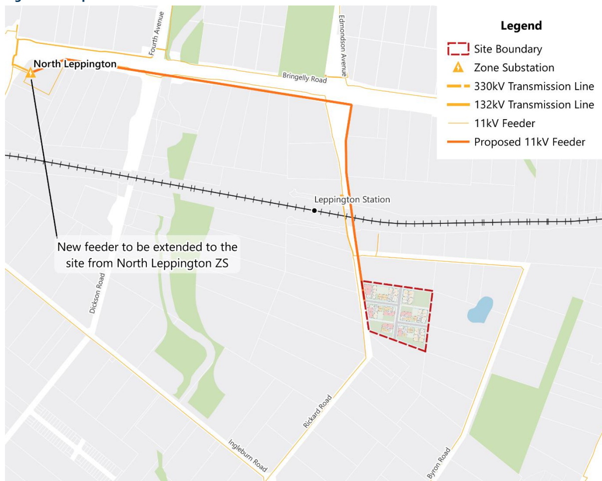
Figure 8 - Proposed Electrical Infrastructure
